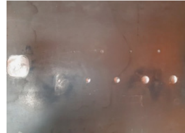
ECA custom probe on various round bottom holes over a 30 mm rubber tile
