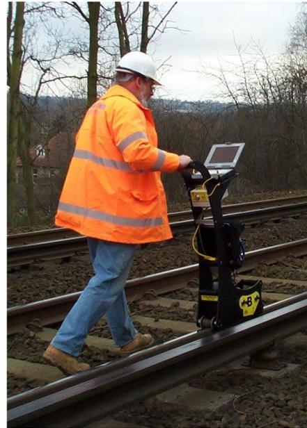
ACFM® was originally developed for use in the oil and gas industry as a technique for detecting and sizing surface-breaking defects with minimal surface preparation. It is now used in a wide variety of industries as an alternative to magnetic particle or dye penetrant inspection. In the rail industry it is being used to inspect axles, wheels, bogies and rails, where it is able to complement ultrasonic inspection:
