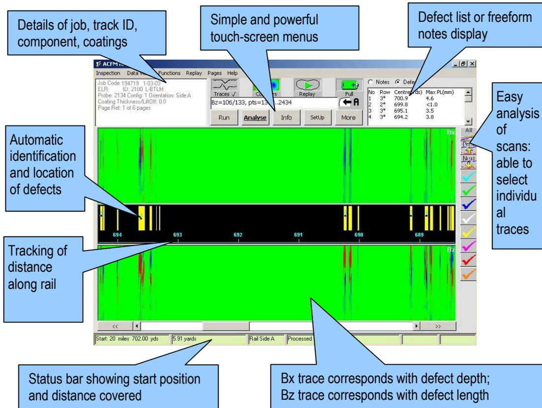
In 2011, TSC joined the INTERAIL consortium which was funded by the EU to bring together Universities and technology companies with the aim of formulating inspection technologies which could inspect rail tracks at high speeds. The prototype ACFM® system produced during the project was capable of detecting RCF oriented defects 12mm x 2mm in size at 80kph.
