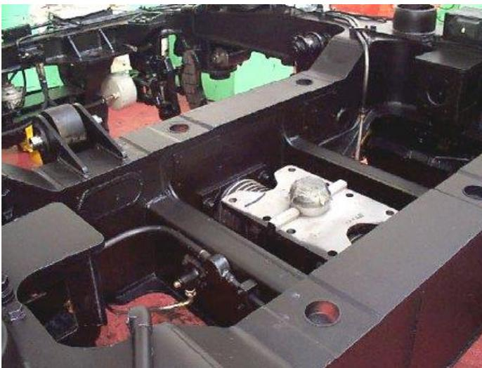
Bogies contain a large number of welds, usually of short length and quite often difficult to access. Such welds are traditionally inspected using MPI, but this involves removing dirt and paint prior to inspection, and reapplying the paint afterwards. This time-consuming operation is avoided with ACFM. To inspect the welds with ACFM, a variety of probes with differently angled or lengthened heads are used, depending on access.
