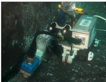
UWILDs are often highly scrutinized by supervising surveyors, as the inspector is the only one with direct access to the structure being inspected. Traditionally this will be the inspecting diver, who needs to be certified by a regulatory body, which can be expensive and increases the risk factors involved. Safety concerns around divers in the water is now being answered by the use of ROVs and robotic crawlers.
