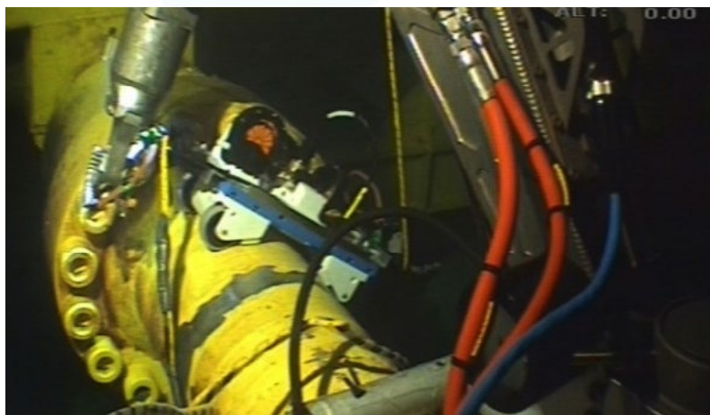
Figure 1 (above) ACFM® scanning pipeline at 1100m depth.
