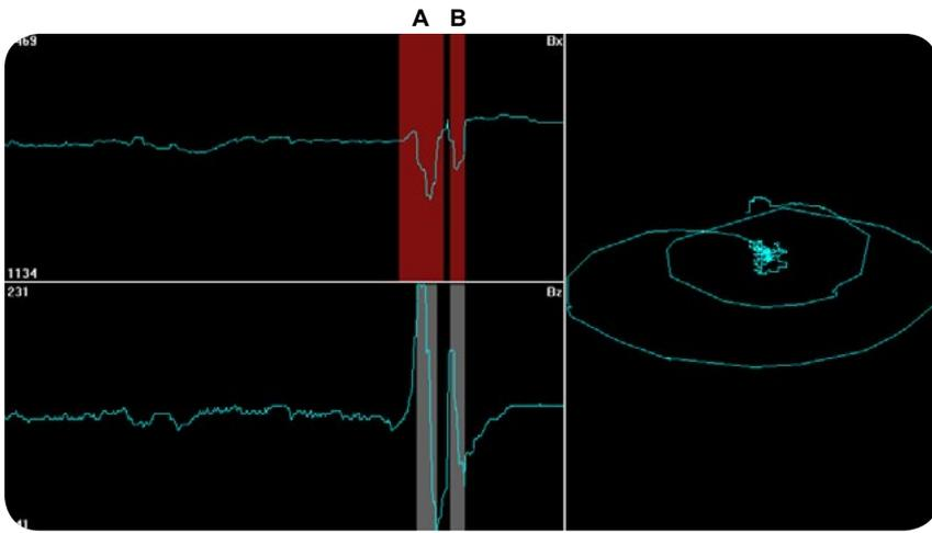
Thames Bridge, built in 1867: ACFM® signals from 2 defects on a bridge weld (left) with MPI indications from the same defects (right). Defect **A** was 20 mm long by 3.9 mm deep; defect **B** was 10 mm long by 3.0mm deep.
