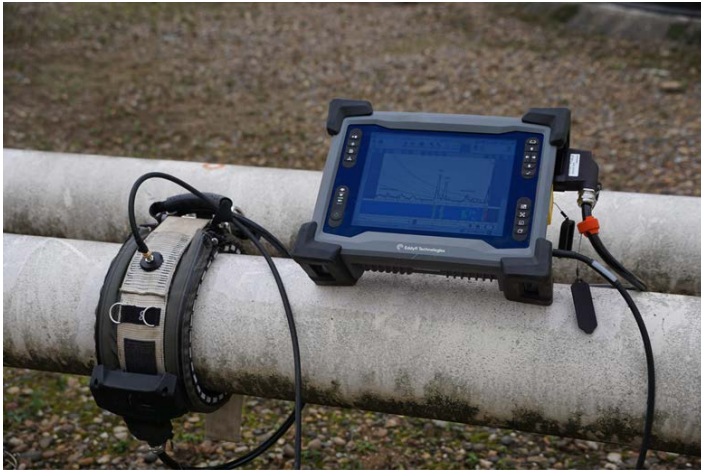
Figure 3: Sonyks instrument with the Piezo tool on site
